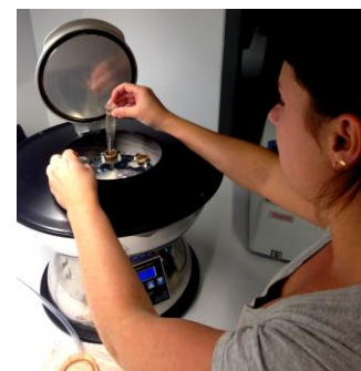
Anna Murphy, wine laboratory manger, loads a sample into the centrifuge for clarifying.
