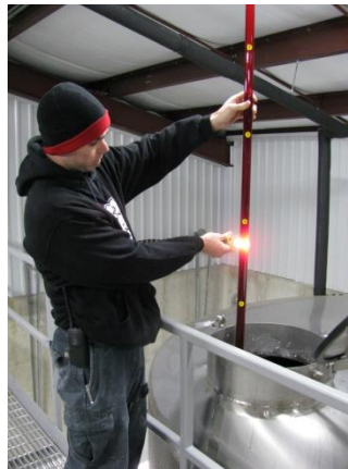
LIQUA-CORE Core Sampler for viewing and measuring settled solids in wine and beverage tanks. Model L-20208
